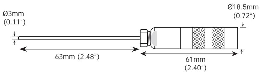
Integral Remote Temperature Probe Dimensions
