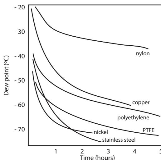
All materials are permeable to water vapor, as the water molecule is extremely small compared to the structure of solids, even when compared to the crystalline structure of metals. The graph above shows the dew point inside tubing of different materials when purged with very dry gas, where the exterior of the tubing is in the ambient environment.
