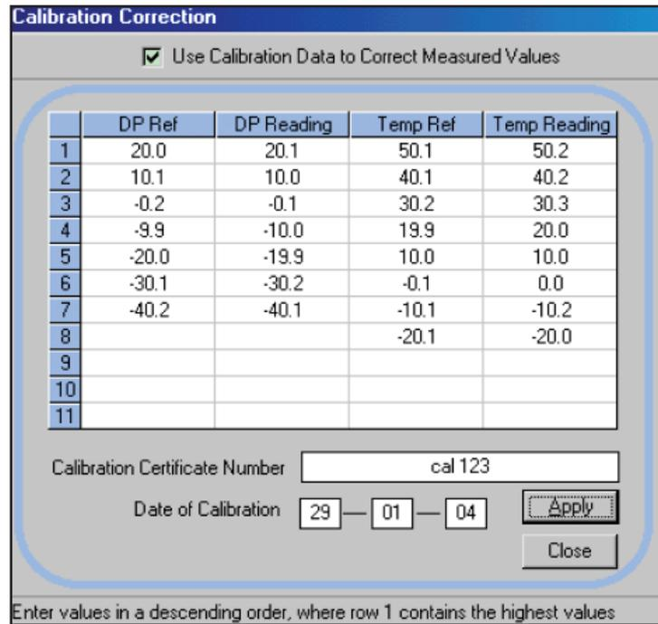
Figure 11 Calibration Correction Window
